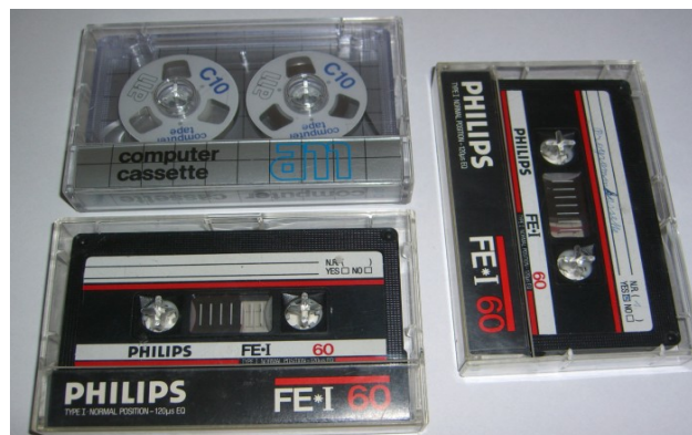
Figure 8. Tapes Used for Evaluation of Migration Tool. Upper left corner: C10 computer cassette; lower left and right Philips FE-I 60 normal position audio tapes.
