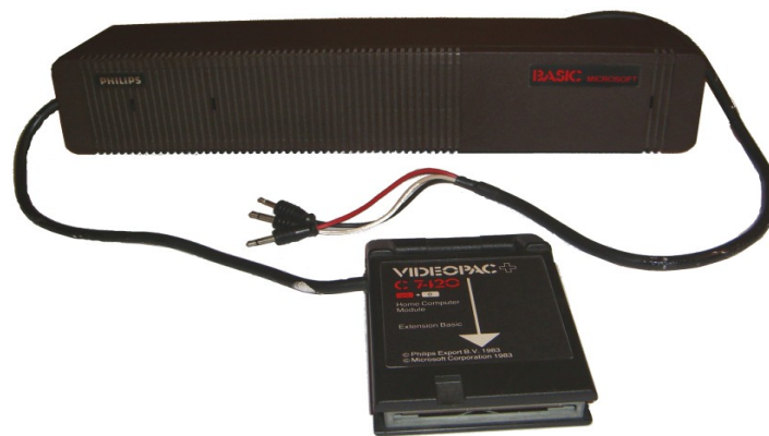
Figure 2. Philips Videopac+ C7420 Home Computer Cartridge: The cartridge plugs into the system at the front, connecting to the main case that holds the additional CPU and memory in the back. The connectors for loading/saving data to an audio system (red, white and black cables for microphone, headphones and remote control) are attached to the main case.
